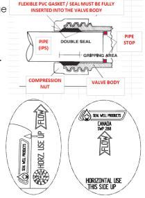
**#6** - Slide the outlet compression nut followed by the gasket onto the discharge pipe from the check valve until it covers the marking from step 3, position the discharge pipe into the valve body ensuring it bottoms out.
