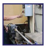
Hydrant being assembled using a custom made power torque wrench complete with electric eye. This is what ensures proper torque with precise alignment of drain port on every hydrant.
