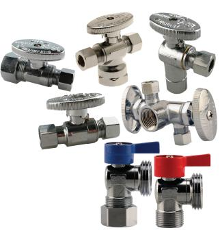
Standard compression valves can be used to make connections between Copper, Brass, Aluminum, Plastic, CPVC & PEX tubing. Not recommended for use with steel tubing. They are designed for use with tube manufactured to CTS-OD copper tubing sizes (outside diameter controlled).
