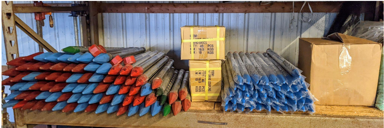
Sandpoints, couplers and drive caps awaiting shipment from Union, Kentucky to Lusaka Zambia. February 10, 2022
