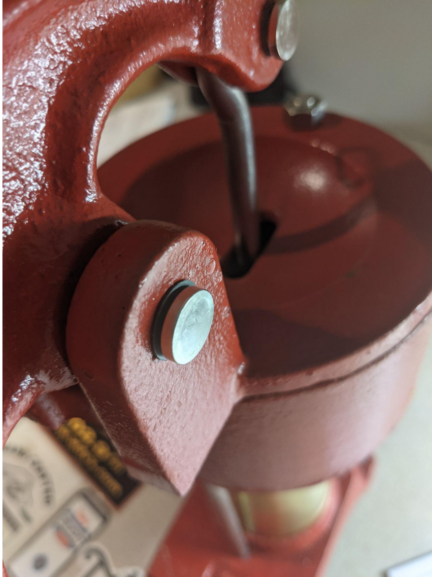
Close up of the Indiana pump. Note polymer flange bearings and stainless steel clevis pins. August 12, 2021.
